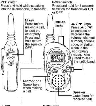
L key Press to turn the display backlight ON. Press and hold to lock the MODE key and Power switch.
