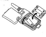
4 Replace the battery cover, making sure the battery cover latch locks in place.
